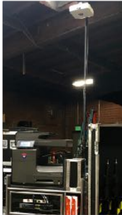
Place Access Point on built in stand, raise the stand as high as you can. This AP gets
